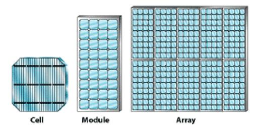
SOLAR RELATED EQUIPMENT: Items including a solar photovoltaic cell, module, or array, or solar hot air or water collector device panels, lines, pumps, batteries, mounting brackets, framing and possibly foundations or other structures used or intended to be used for collection of solar energy.
